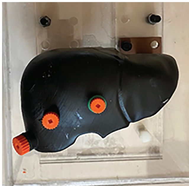
Figure 1. View of the liver phantom inside the water tank. The figure shows the liver phantom placed inside a water tank. The filling caps, from left to right, correspond to the normal liver, small tumor, and large tumor compartments, respectively
